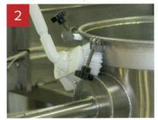
This adjustable water-fed brush with soft bristles is ideal for cleaning stainless steel equipment. Adjustable for ease of cleaning vertical surfaces and cleaning high areas.
