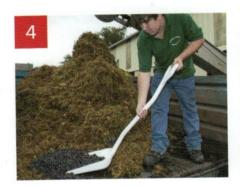
Ergonomic shovels exert less pressure on the operator's back, making it easier to scoop.
