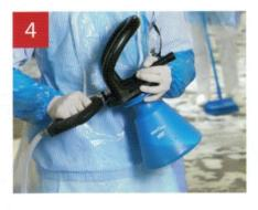
Foam sprayers are perfect for cleaning sanitary and small processing areas. Foam is applied without aerosols at normal water pressure.
