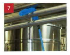
This flexible brush can be bent into shape as required and is effective for cleaning external pipe surfaces. A soft version of this brush is also available for moving dust.
