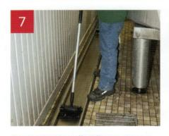
Rounded brushes offer effective cleaning for drains. We recommend the use of a specific colour for bungs and drains in order to avoid contamination.
