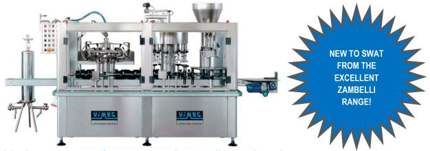
Triblock consisting of Rinsing Machine, Filler and Corker
